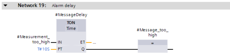
Fig. 8.23 Example of IEC timer functions in the function block diagram
