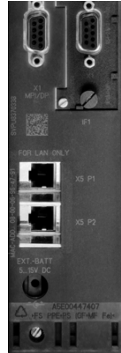
Fig. 2.9 The bus connections on a CPU 416-3 PN/DP
