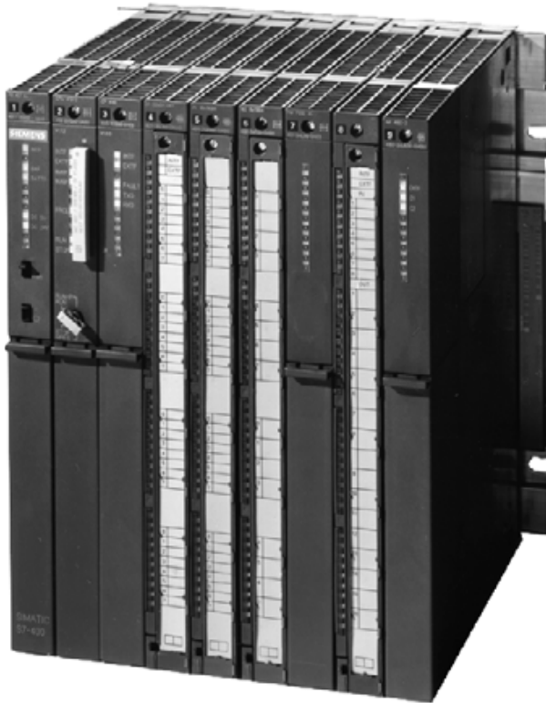
Fig. 2.1 S7-400 programmable controller in a UR2 rack
